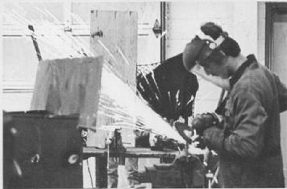
J. R. Kiner, senior, demonstrates how to use a disk sander in welding. He wears special protective clothing while doing this so not to burn himself or his clothing. A face guard is also worn to keep the sparks from hitting him in the face.
